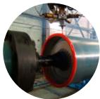
It uses 3 components which levels can be varied to produce polyurethane rolls from 65 Shore A up to 95 Shore A. The rapidly reacting 3 component system is poured onto a rotating core and is built up in a series of passes to the specified diameter. In some cases rollers can be machined to exact specifications after 1 hour of room temperature postcure, this depend on material hardness and roll size.
